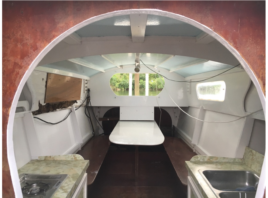
Looking Rearwards, past bunks, into galley, dinette area with solar powered fridge in floor under table - cabin side needs replacement
