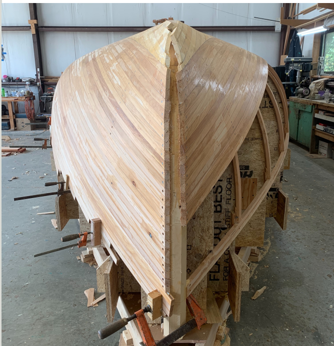
Our boatbuilding shop finishes planking the port side of the 22' racing catboat we're building this fall and winter. It is a new design that will debut in 2021.
