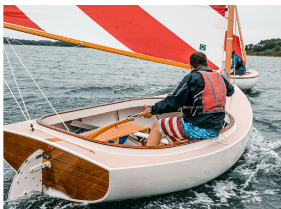
A view of the varnished transom, redesigned rudder, and streamlined cockpit on the 2021 14' Racing Catboat. Pleasant Bay, MA.
