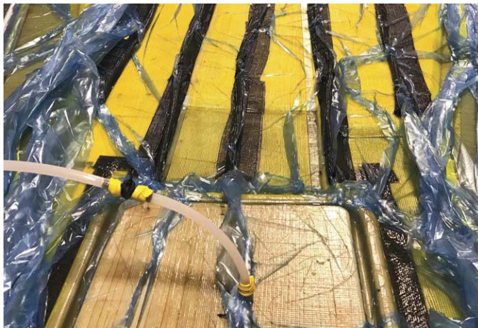
Front Street Shipyard uses a vacuum-bag process to infuse resin into the carbon fiber lay-up of a boat deck. Carbon fiber has an excellent strength-to-weight ratio, said the company's president, JB Turner. Image courtesy Front Street Shipyard.
