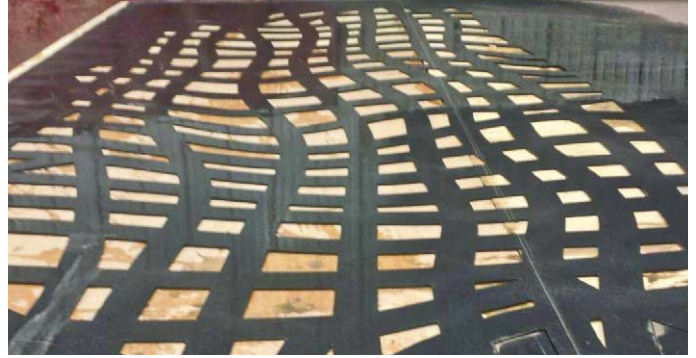
Nautilus Marine used waterjet technology, blasting 50,000 pounds of pressure per square inch, to cut intricate lattice work for Foggy , a 74' German Frers-designed daysailer built by Brooklin Boat Yard for architect Frank Gehry. Image courtesy Brooklin Boat Yard.
