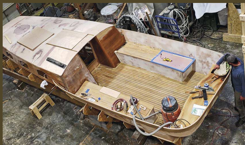
Left: Hewes & Company cut pieces for the cockpit and house mold for Brooklin Boat Yard's construction of a 44-foot coastal racing/day boat. Right: The completed construction of that same cockpit and house made from the mold. Photos courtesy Hewes & Company
