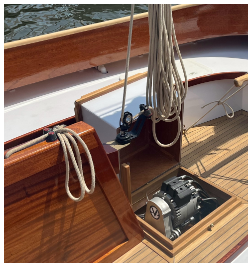
Inboard electric OceanVolt engine in a Arey's Pond 19' Caracal launched this summer.
