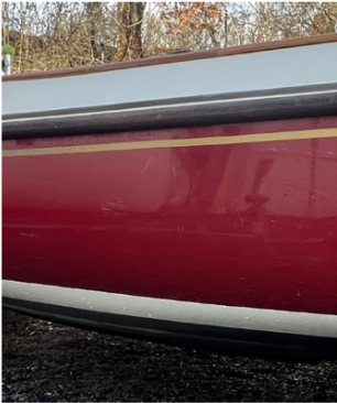
This is an example of a vessel with a red hull, white bootstripe, and black bottom paint.
