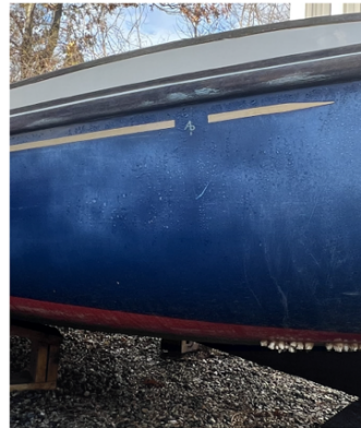
This is an example of a blue hulled vessel whose gel coat has oxidized over time.
