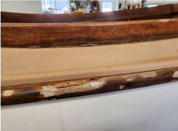
Figure 9: This depicts Cetol that is peeling back that could be stripped and the underlying teak left natural.
