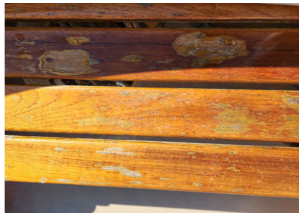
Figure 8: This is an example of varnish that has failed, designated by the yellowed varnish and bare wood. This would be considered more than a simple maintenance coat.
