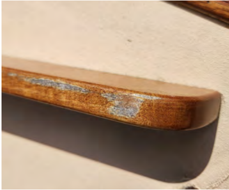
Figure 6: This is an example of a maintenance coat that warrants some buildup in spots where the varnish has failed and the wood is exposed.
