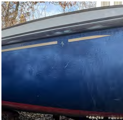
Figure 1: This is an example of a blue-hulled boat with gel coat that has oxidized over time.
